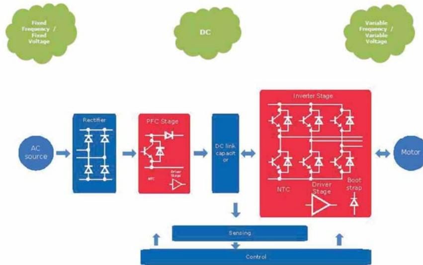
Typical solution for Inverterized Appliance
