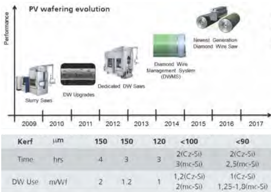
Fig. 1: Changes in kerf, cutting time and wire consumption resulting from the changeover from slurry process to a dedicated diamond wire saw, taking the example of the DS271 and the DW288 Series 3 (source: Meyer Burger(Switzerland) AG).
