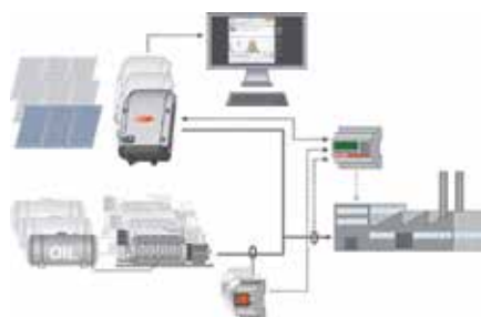
Picture 1: SE HRPIC Fronius PV Genset.
