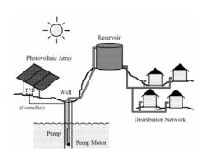
people "at the Bottom of the Pyramid", the bare need is Clean Drinking Water, in smaller quantities. If a small capacity 12V DC Diaphragm type submersible pump is directly connected to Solar PV Panel, without Battery, it can deliver from about 1000 liters to 2000 liters/day depending upon the depth from which it is pumped out. If 3-4 such systems with storage water tank are setup in a rural cluster, it can provide enough clean drinking water for a rural cluster. Cost for a single
